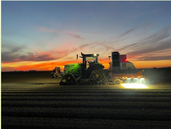
Shown above is the Carbon Robotics Laser Weeder removing weeds without herbicides.
